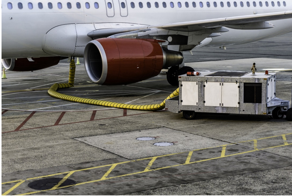
Figure 4.4 Ground Cart Combined Air-Conditioning and Power Unit
