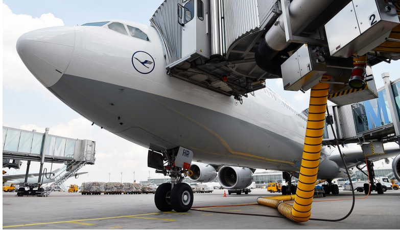
Figure 2.3 Example of a Jet-bridge Mounted PCA Unit and Yellow Hose Supplying Air to the Aircraft Parked at the Gate (Source: Munich Airport, retrieved from https://www.munich-airport.com/a-fresh-breeze-thanks-to-pca-1229006# )
