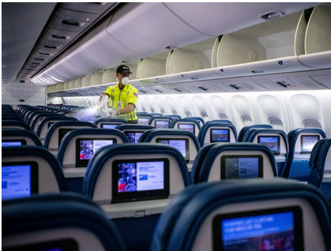
Figure 9.3 Electrostatic Spraying in an Aircraft Cabin
