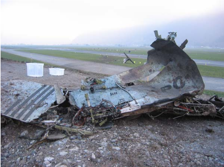
Final position of wing main- spar / fuel tank section
