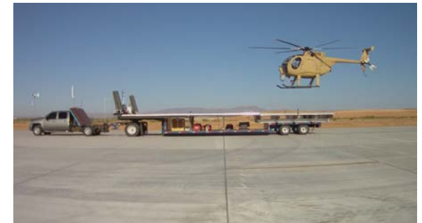
H-6U landing to trailer
