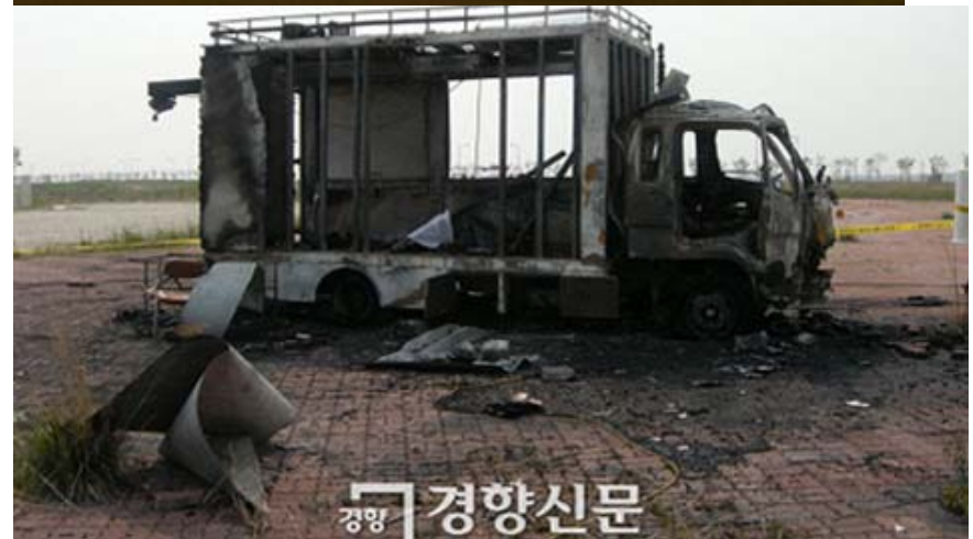
RF environment caused Camcopter loss of control, impacted GCS, and one fatality
