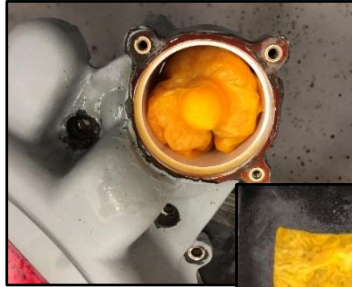
FOD identified as wadded-up oil absorbent pad
