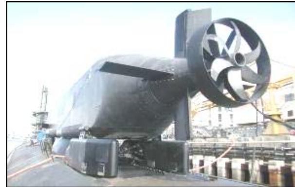
Design of Flow Control Device to Eliminate Rudder Fatigue Cracking Due to Unsteady Flow and Loads
