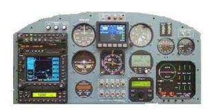
Modern Avionic and Electronic systems can, if properly installed, provide additional situational awareness, easier navigation and additional safety. Good examples are AOA indicator, stall warnings, flight displays, GPS and collision warning systems.
